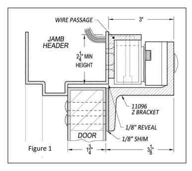
For wood jambs or clad door framing, the structure must be capable of carrying the holding force generated by the magnet. The use of reinforcing material or bolting Through the header may be required.
