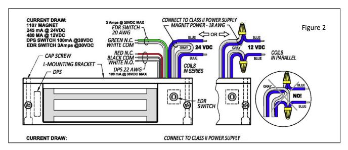
Connect the 20 AWG Normally Closed white and green wires to the lock controller.
