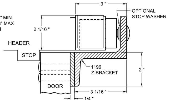
Z-BRACKET IS THRU-BOLTED TO DOOR USING THE Z-BRACKET TEMPLATE PATTERN. THE SCREWS PASS THROUGH THE SHIM.
