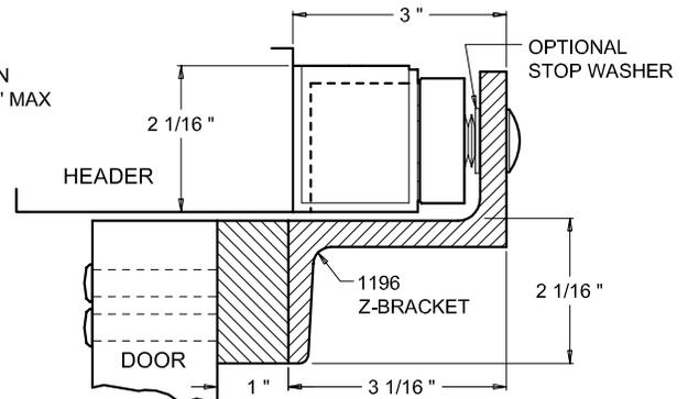
SPACER BLOCK IS THRU BOLTED TO DOOR USING THE BLOCK THRU BOLT PATTERN. Z-BRACKET IS THEN MOUNTED TO THE BLOCK, BY MEANS OF THE Z-BRACKET SCREWS AND THE TAPPED HOLES IN THE BLOCK.
