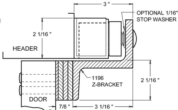
Z-BRACKET IS THRU-BOLTED TO DOOR USING THE Z-BRACKET TEMPLATE PATTERN. THE SCREWS PASS THROUGH THE SHIMS. SHIM STACKS OF 1/2" TO 7/8" USE LONGER 1 1/2" SCREWS FURNISHED WITH SHIMS.
