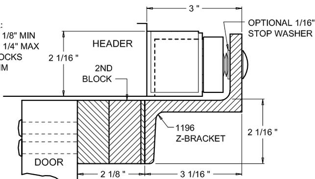
THE SECOND SPACER BLOCK IS THRU BOLTED TO DOOR USING THE BLOCK THRU BOLT PATTERN, WITH THE SCREWS PASSING THROUGH THE FIRST BLOCK. Z-BRACKET IS THEN MOUNTED TO THE SECOND BLOCK, USING THE TAPPED HOLES, WITH THE APPROPRIATE LENGTH SCREWS PASSING THROUGH THE SHIM.
