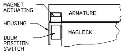
THE DPS SWITCH IS ALWAYS LOCATED ON THE WIRING ENTRY SIDE.
