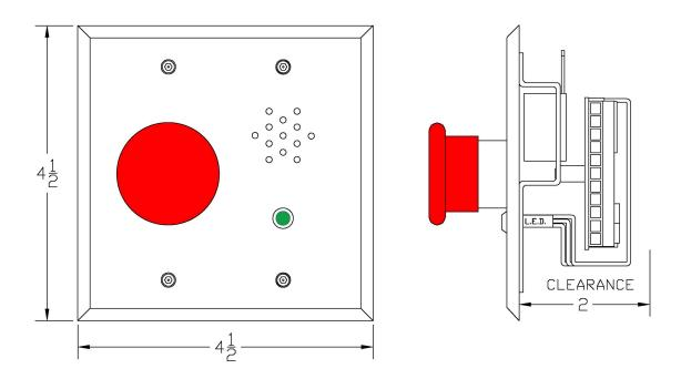
**7281-EAXMP23** Door Alarm Module on 2-gang stainless steel plate with LED and sounder. Includes 1-9/16" dia. momentary exit push button (1-N.O. & 1-N.C. contacts).
