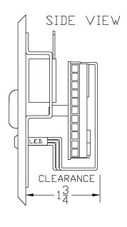
**7281-EA-K332** Door Alarm Module on a 2-gang stainless steel plate with LED and sounder. Includes electrical key switch with DPDT maintained contacts, The key is removable in both positions.
