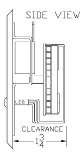
**7281-EA** Door Alarm Module on 1-gang stainless steel plate with LED and sounder.
