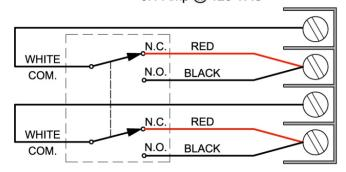
NOTE: PULLING THE HANDLE RELEASES THE SWITCH SO THAT CONTACT DESIGNATIONS SHOWN ARE TRUE WHEN HANDLE IS PULLED.
