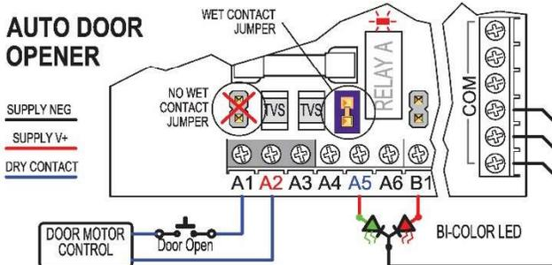
When the relay is energized the door OPEN request circuit is enabled. The LED turns green to indicate that the door may be opened. When the relay is not energized, the door OPEN request circuit is interrupted. The red LED shows that the door is not available for access.
