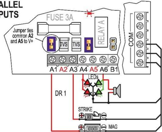
Use Parallel connections to operate multiple devices from a single DPDT relay output. Wet contact jumpers eliminate having to connect relay common back to V+ out terminals. Though fused for 3 Amps, do not exceed 2 Amp holding current per set of contacts to ensure optimum service life.
