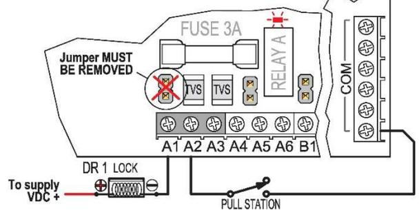
Some installations require that the lock relay switches the lock ground lead. Relay common must be wired to the ground and the WET CONTACT jumper must be removed to prevent a short circuit and possible damage to the board.
