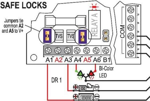
The convention for Dortronics controllers is fail safe - the relay energizes to lock the door. Connect mag locks to the normally open contacts. Connect other lock types for the desired operation.
