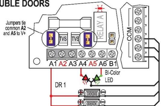
For double doors, connect locks in parallel to the fused contacts. The LED for lock status indication can be connected to the second set of contacts. Current for both locks should not exceed 1.5 Amps for maximum reliability.
