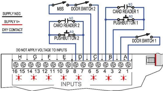
Two or more normally open **dry contact** switches can be connected in parallel at any input. Similarly, Door Position Switches and Magnetic Bond Sensors (or other sensor outputs) can be connected in series as long as the contacts are dry.
