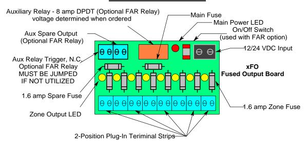
Input: 12 or 24 VDC, 90mA with Auxiliary Relay installed
