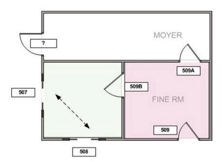
The following chart indicates the relationships between doors. Swinging doors are to be secured with maglocks. The circuit to open the automatic sliding doors will be shunted by the Interlock Controller when they are not available for access.
