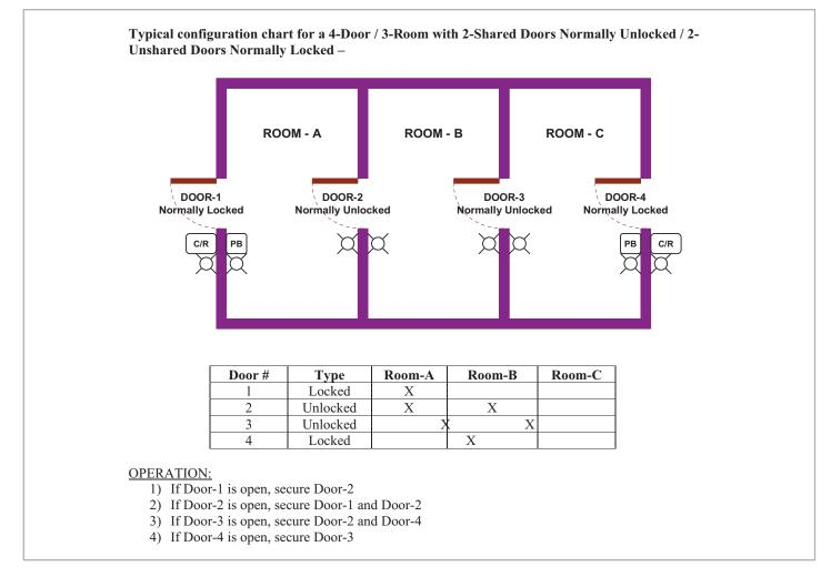
Doors 'shared" between rooms generally inhibit all other doors in both rooms. Since these doors are already within the secure area, they can sometimes be specified as normally unlocked to increase traffic flow.
