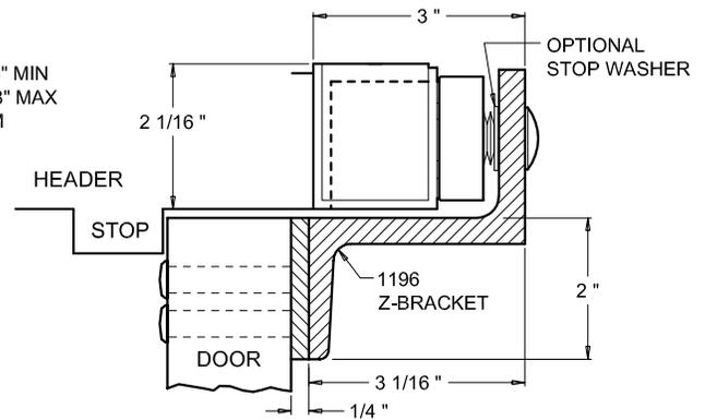
Z-BRACKET IS THRU-BOLTED TO DOOR USING THE Z-BRACKET TEMPLATE PATTERN. THE SCREWS PASS THROUGH THE SHIM.
