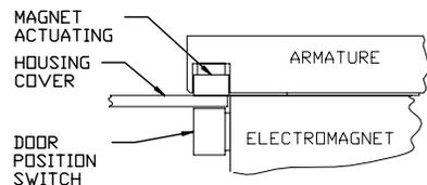
MAY BE AT EITHER END OF ELECTROMAGNET, AND ON EITHER LOCK JAMB OR HINGE JAMB END.
